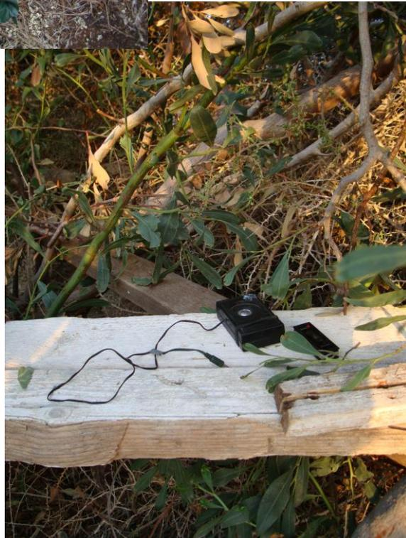
Mini tape lure equipment with device of tape and loudspeaker and a battery for a few hours
