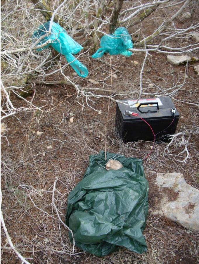
Tape lure with loudspeakers, device with a tape and a battery
